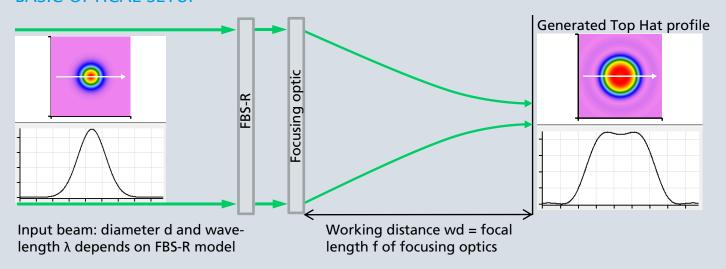
FBS-R beam shaper in combination with any focusing optic and a collimated single mode Gaussian beam (TEM $_{00}$  with M $^2$  of 1.4 or better) delivers a homogeneous Top Hat profile. This Top Hat profile is generated in the focal plane of the focusing optic. The size of the generated Top Hat spot depends on the focal length f, the input beam diameter d (@1/e $^2$ ) and the wavelength  $\lambda$ . The Top Hat diameter (@1/e $^2$ ) is approximately 2 \*  $\lambda$  \* f / d.
