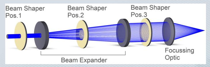
Pos. 1: FBS-R can be installed in front of a beam expander/telescope into the beam. Advantage of this option is scaling of the spot size in focal plane by changing the magnification of the beam expander.
