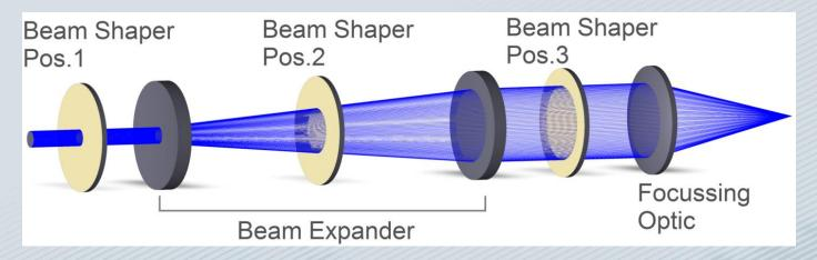
Pos. 1: FBS can be installed in front of a beam expander/telescope into the beam. Advantage of this option is scaling of the spot size in focal plane by changing the magnification of the beam expander.
