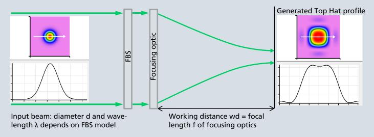
FBS beam shaper in combination with any focusing optic and a collimated single mode Gaussian beam (TEM $_{00}$  with M $^2$  of 1.4 or better) delivers a homogeneous Top Hat profile. This Top Hat profile is generated in the focal plane of the focusing optic. The size of the generated Top Hat spot depends on the focal length f, the input beam diameter d (@1/e $^2$ ) and the wavelength  $\lambda$ . The Top Hat width (@1/e $^2$ ) is approximately 2 \*  $\lambda$  \* f / d.
