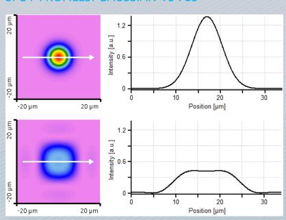
Above: Spot profile of a focused Gaussian beam in the focal plane (left) and the corresponding line scan (right).
