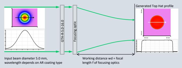
GTH-R-5.0-16.0 beam shaper in combination with any focusing optic and a collimated Gaussian beam dia. 5.0 mm (@ $1/e^2$ ) delivers a homogeneous Top Hat profile. This Top Hat profile is generated in the focal plane of the focusing optic. The size of the generated Top Hat spot depends on the focal length f (= working distance).
