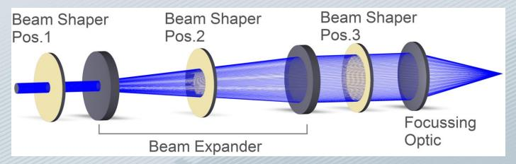
Pos. 1: GTH-R-5.0-16.0 can be installed in front of a beam expander/telescope into the beam. Advantage of this option is scaling of the spot size in focal plane by changing the magnification of the beam expander. The diameter of the generated Top Hat depends on the focal length f of the focusing optic as well as on the magnification m of the beam expander (m = beam diameter behind / beam diameter in front of expander). The beam expander can also be used
