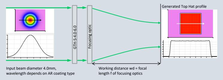
GTH-S-4.0-6.0 beam shaper in combination with any focusing optic and a collimated single mode Gaussian beam dia. 4.0 mm (@ $1/e^2$ ) delivers a homogeneous Top Hat profile. This Top Hat profile is generated in the focal plane of the focusing optic. The size of the generated Top Hat spot depends on the focal length f (= working distance).
