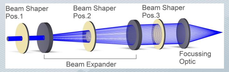
Pos. 1: GTH-S-4.0-6.0 can be installed in front of a beam expander/telescope into the beam. Advantage of this option is scaling of the spot size in focal plane by changing the magnification of the beam expander. The width of the generated Top Hat depends on the focal length f of the focusing optic as well as on the magnification m of the beam expander (m = beam diameter behind / beam diameter in front of expander). The beam expander can also be used reverse to reduce
