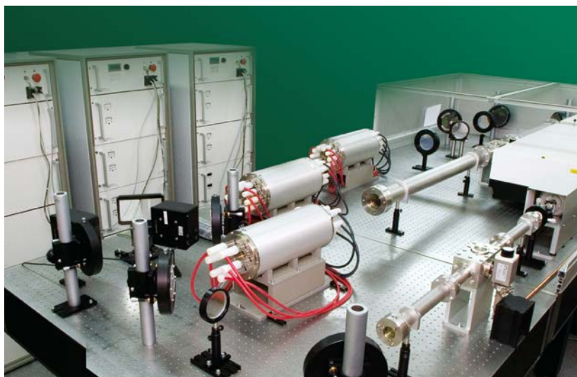
160 J @ 1053 nm MM laser system
