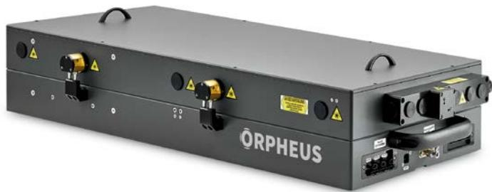
ORPHEUS-TWINS consists of two independently tunable optical parametric amplifiers (OPAs) in a compact footprint. The OPAs are optically synchronized and provide simultaneous outputs. Integrated into a single housing, both OPAs share the same white-light seed enabling the generation of broadband mid-infrared (MIR) radiation with a passively stable carrier-envelope phase (CEP).
