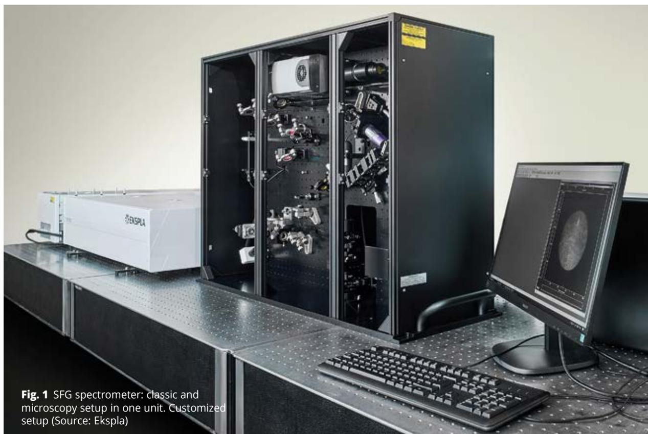
**Fig. 1** SFG spectrometer: classic and microscopy setup in one unit. Customized setup (Source: Ekspla)
