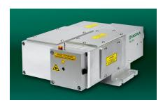
NL200 is a well-proven diode-pumped nanosecond laser for scientific and industrial applications. This laser provides up to 4 mJ at 1064 nm with a variable repetition rate of up to 1 kHz and excellent beam properties like  $\rm M^2{<}1.3$  and pulse energy stability <0.5% RMS. Optionally, the laser can be equipped with harmonics (0.6 mJ / 600 mW at 266 nm, 5th harmonic on request).
